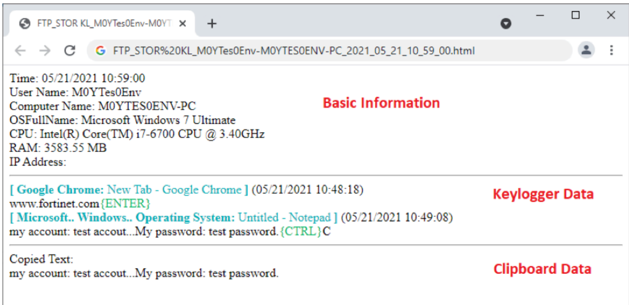
Figure 5.4 – Example of collected keylogger and clipboard data
