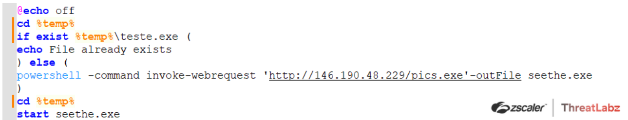
Fig 8. Downloads the final payload “pics.exe” from remote server via Invoke-WebRequest
