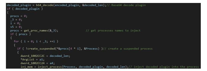
It creates a new suspended process then writes the plugin to the process memory using WriteProcessMemory() and then resumes the injected process.
