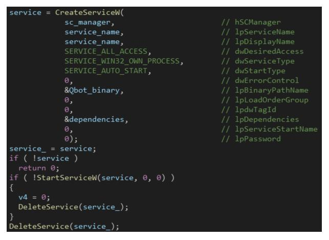
Finally, Qbot deletes the created service and dropped file from the target machine (as it's successfully infected).
