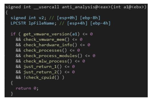
The parent process checks the exit code of this spawned process. If the exit code is not 0, it means that QBot is being analyzed (and so it exits).
