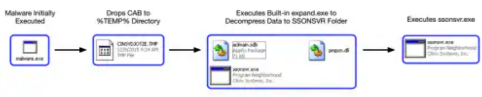
Figure 5 Execution flow of dropper expanding CAB file
