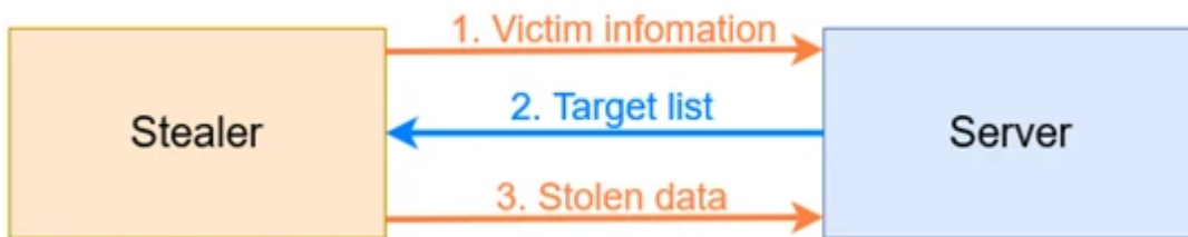
Figure 19: Communication between the server and Fickle Stealer
