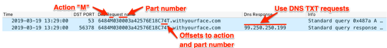
Figure 24. Updated BONDUPDATER's initial beacon and the C2 instructing Trojan to use TXT queries
