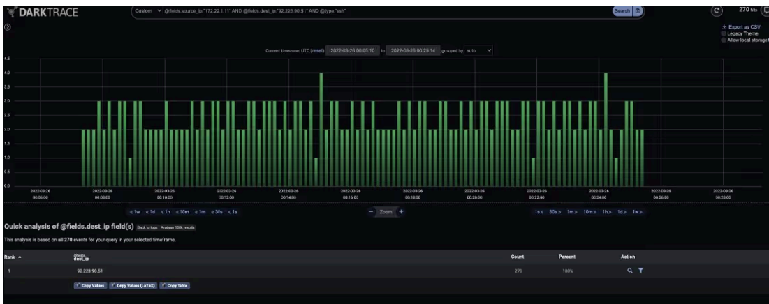
Figure 10: Beaoning SSH connections to a single external endpoint, indicating a potential brute-force attack
