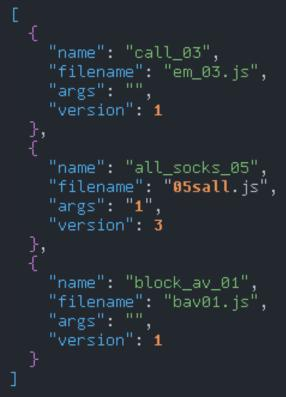
Each entry is parsed, and each filename and args value is passed along for execution by the malware. Detailed analysis of the call\_03 (see Now I See You), all\_socks\_05 (see Click Fraud), and block\_av\_01 (see Block AV Component) components can be found below.
