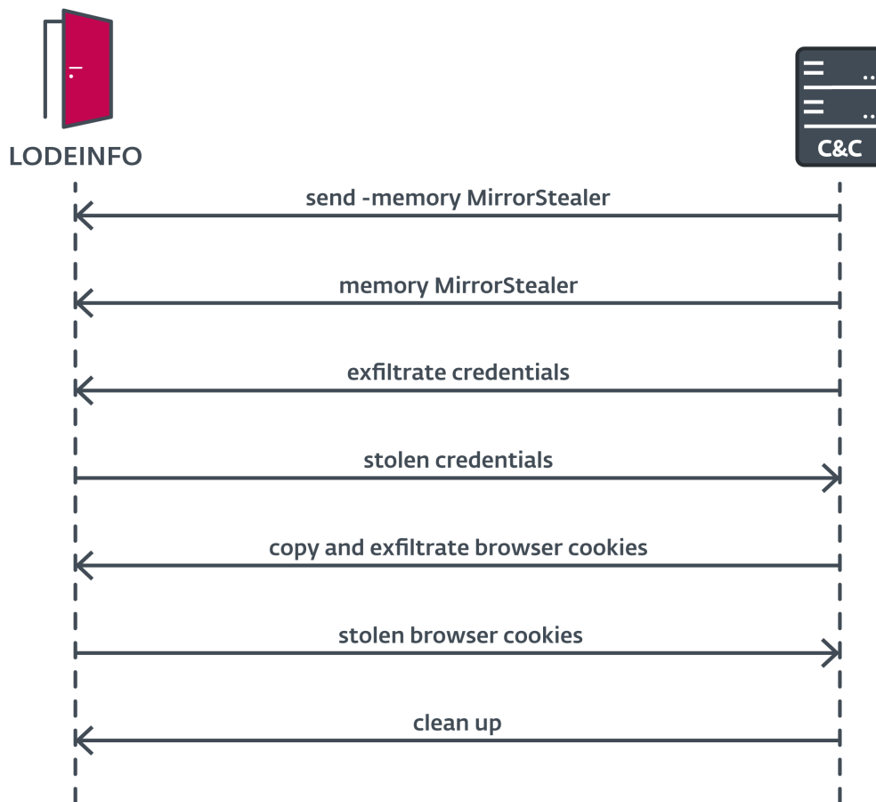
Figure 8. Flow of instructions sent to LODEINFO to deploy credential stealer, collect credentials and browser cookies, and exfiltrate them to the C&C server
