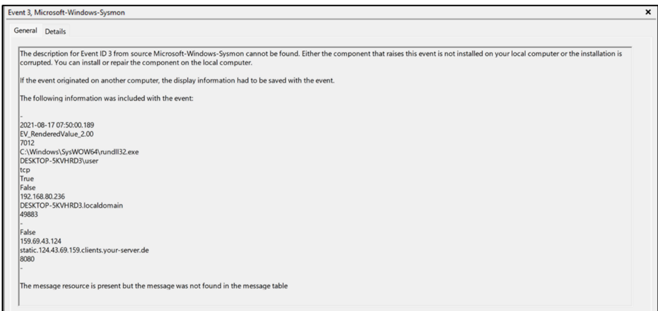
Figure 24 : Malware communicating with C2 Server of 159.69.43.124:8080
