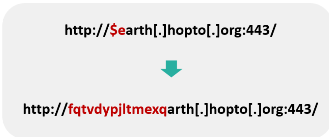
Figure 25. DGA generation using “word” as the placeholder
