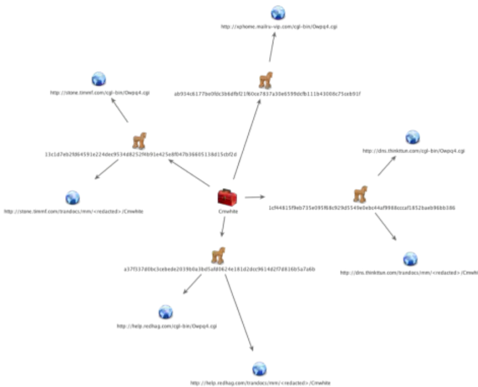
Figure 2. Cmwhite Tools Using "cgl-bin" within HTTP Requests
