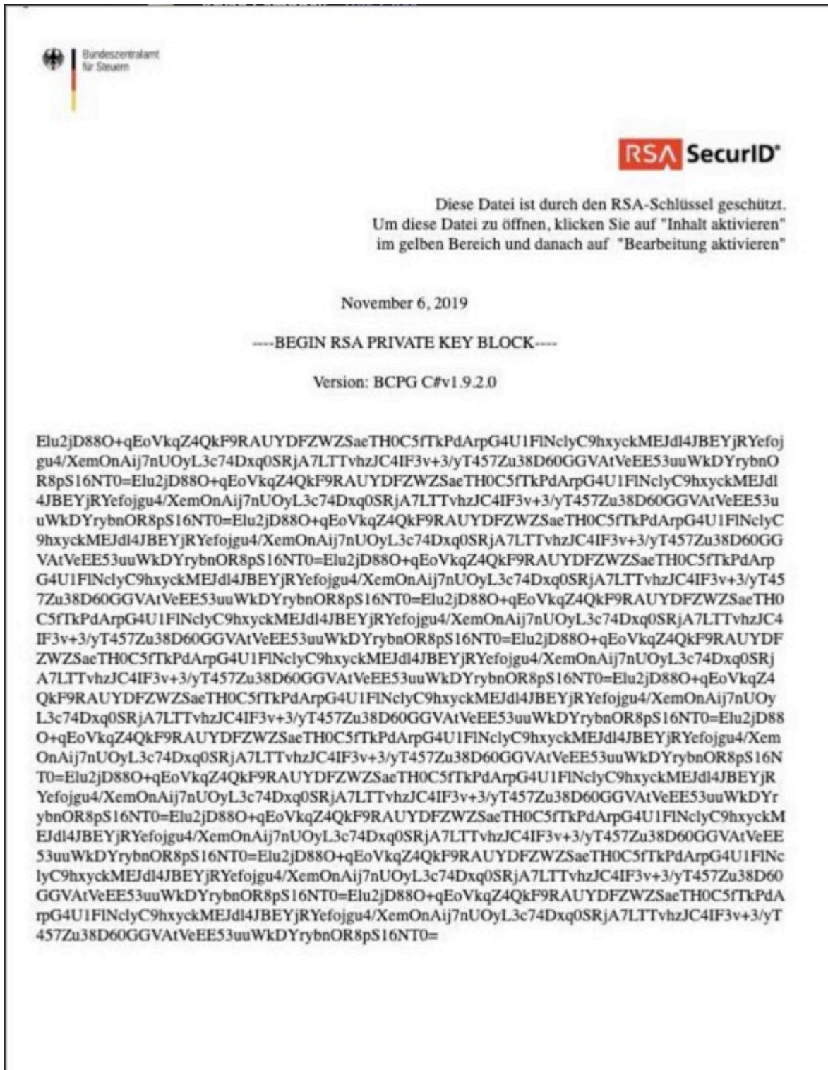
Figure 5: A German-language Microsoft Word attachment which, when opened and the user enables macros, executes a Microsoft Office macro that runs a PowerShell script, which in turn downloads and installs the Maze ransomware payload onto the victim's system.
