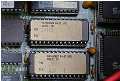
BIOS chips in a Dell 310 that were updated by replacing the chips
