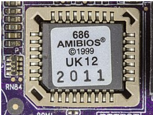
American Megatrends BIOS 686. This BIOS chip is housed in a PLCC package in a socket.
