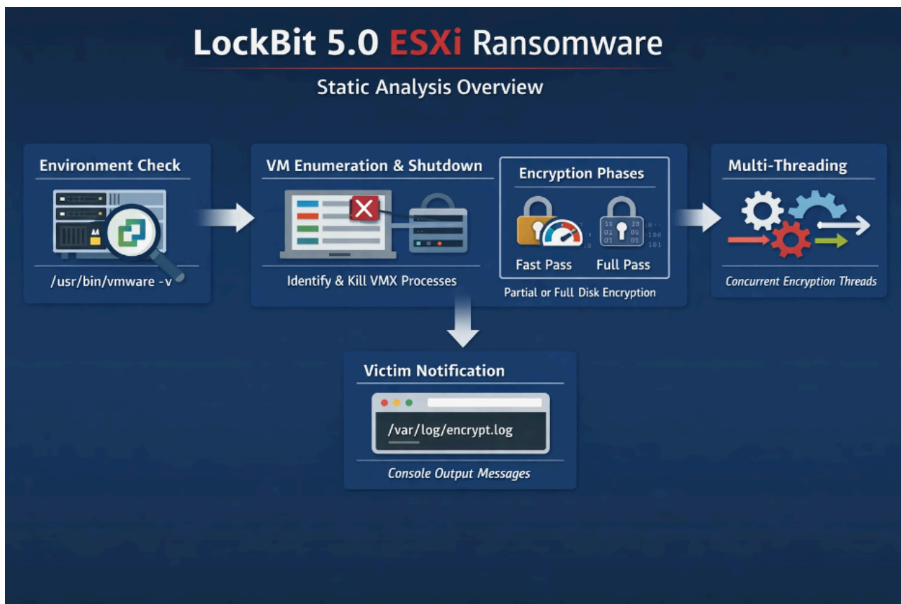
Figure 5. LockBit ESXi execution flow
