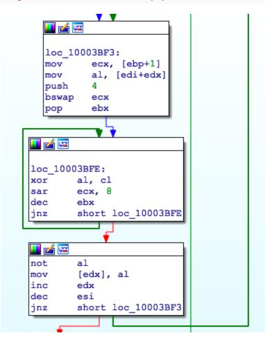
But unpacking a particular sample mentioned earlier , revealed another side of the story . Although the code to load encoded c2 buffer was there , but the coding routine was a clever choice of deception, which feeds a fake encoded c2 buffer , though decoded buffer is a valid http resource , but instead chooses to take the c2 buffer from a plain text value in between the subroutine
