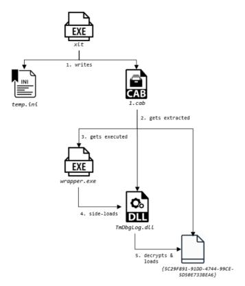
Figure 9: USBCulprit's loading flow, as observed in samples after 2017.
