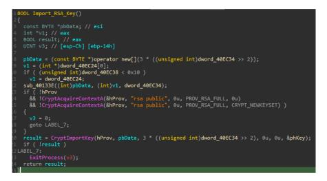
Figure 16. Importing the RSA-2048 public key for encryption
