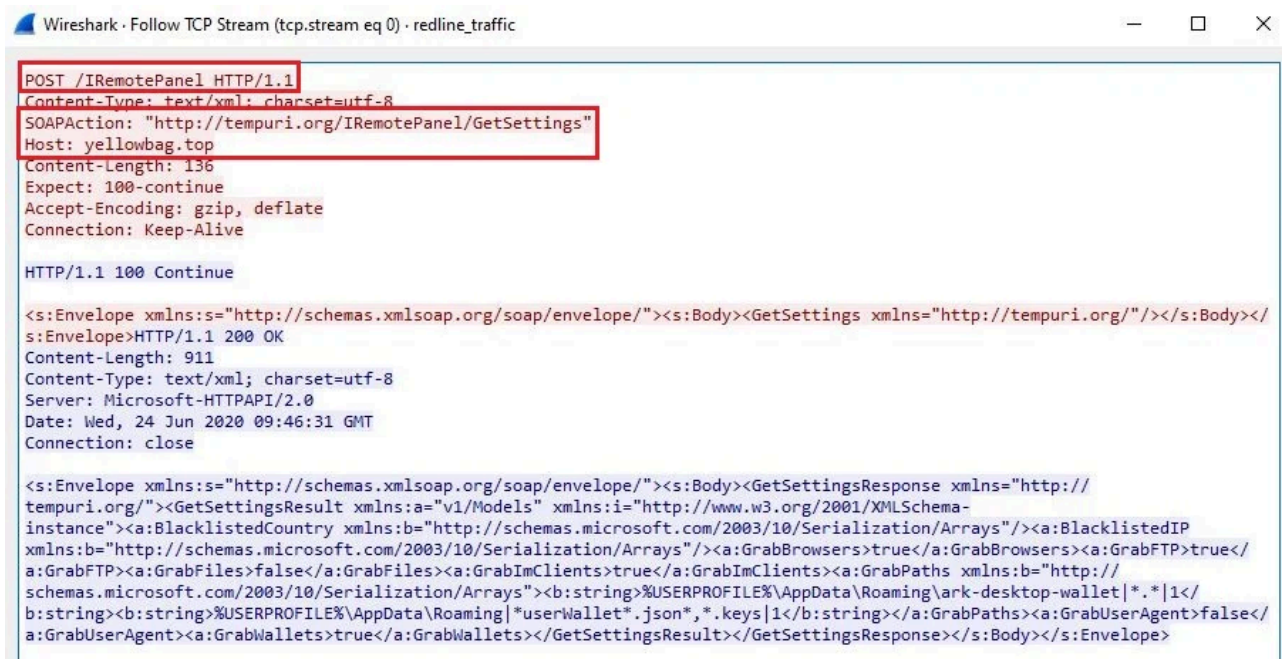
Figure 17: Fetching the client configuration settings.
