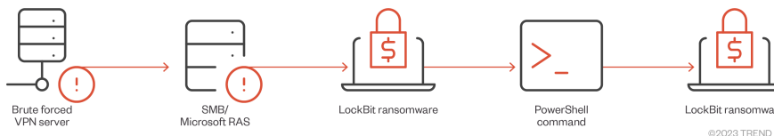
Figure 7. A LockBit 1.0 campaign that used PowerShell Empire to perform command and control after gaining access to the system
