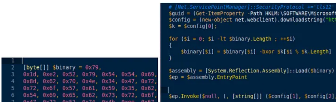
Figure. Binary encoded data inside PowerShell and decryption routine.
