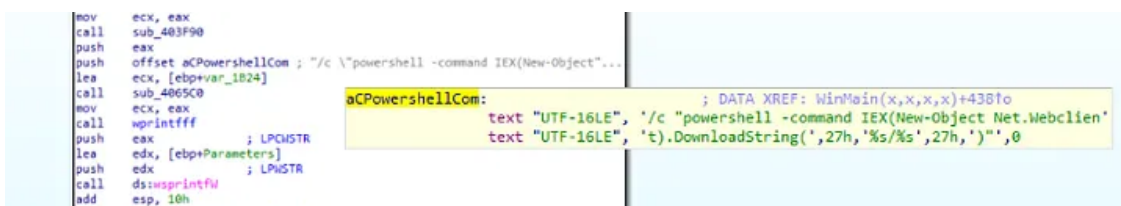
Figure. Command string to retrieve executable PowerShell code
