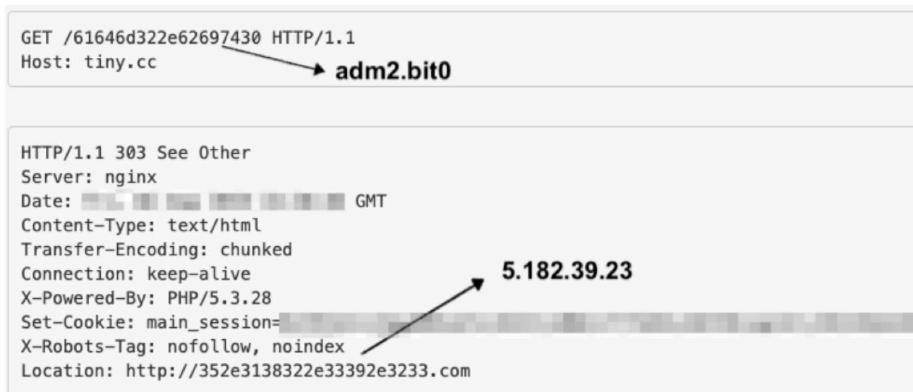
Figure 4: The GET request containing a hex-encoded C&C domain (adm2[.]bit) followed by an HTTP 303 See Other response revealing another hex-encoded DNS server IP Address as a domain.
