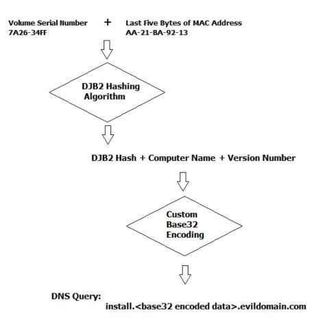
Figure 2. Construction of Installation Beacon
