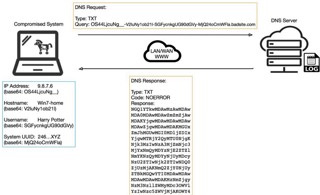
Figure 4. Example C2 DNS query with TXT type response
