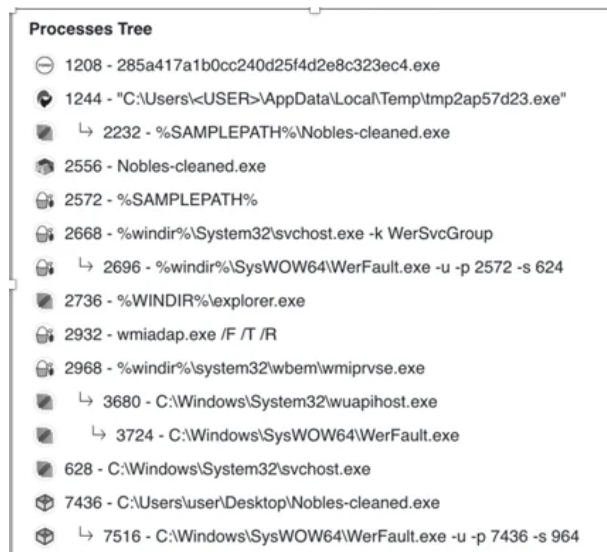
Figure 2 - The variants analyzed do not invoke PowerShell, but continue to leverage Windows Management Instrumentation heavily for core information gathering capabilities from local systems.
