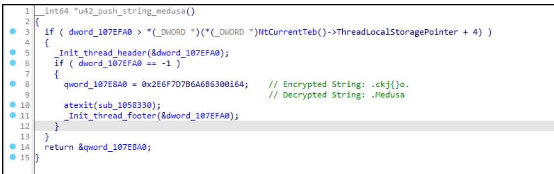
Figure 22. Decompiled view of moving encrypted hex string 0x2E6F7D7B6A6B6300.
