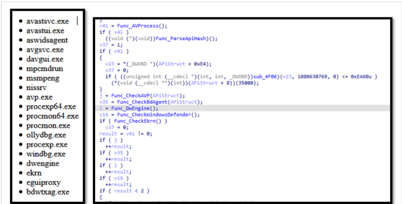
figure 3: Process checking to evade malware lab environment
