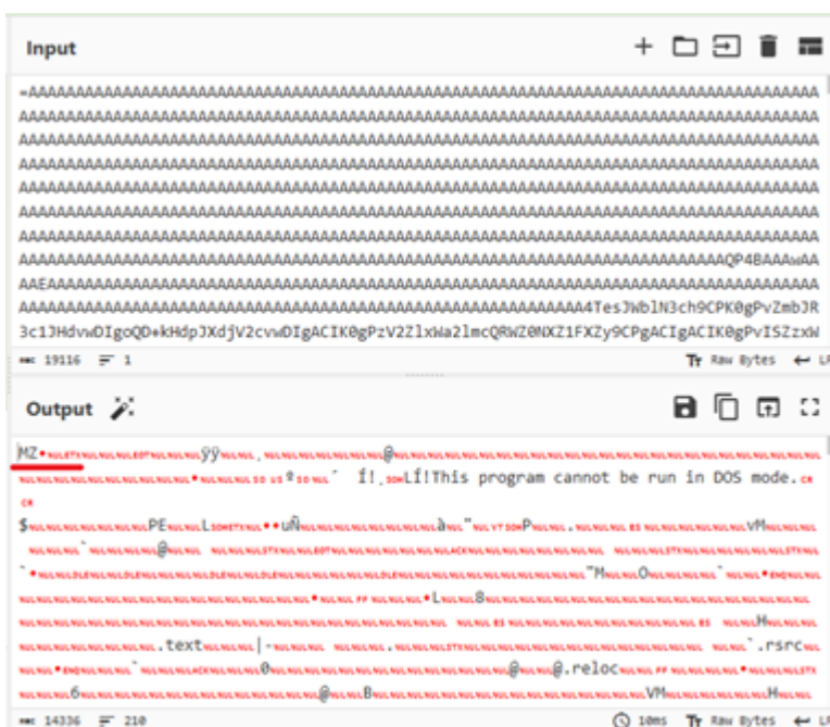
Fig-11: Forming stager-1 by reversing and Base64 decoding
