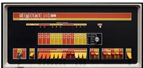
PDP-8/E front panel showing the switches used to load the bootstrap program
