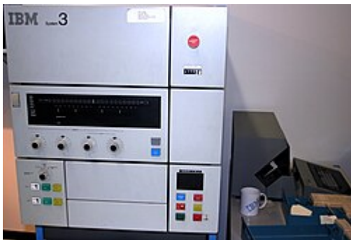
IBM System/3 console from the 1970s. Program load selector switch is lower left; Program load switch is lower right.
