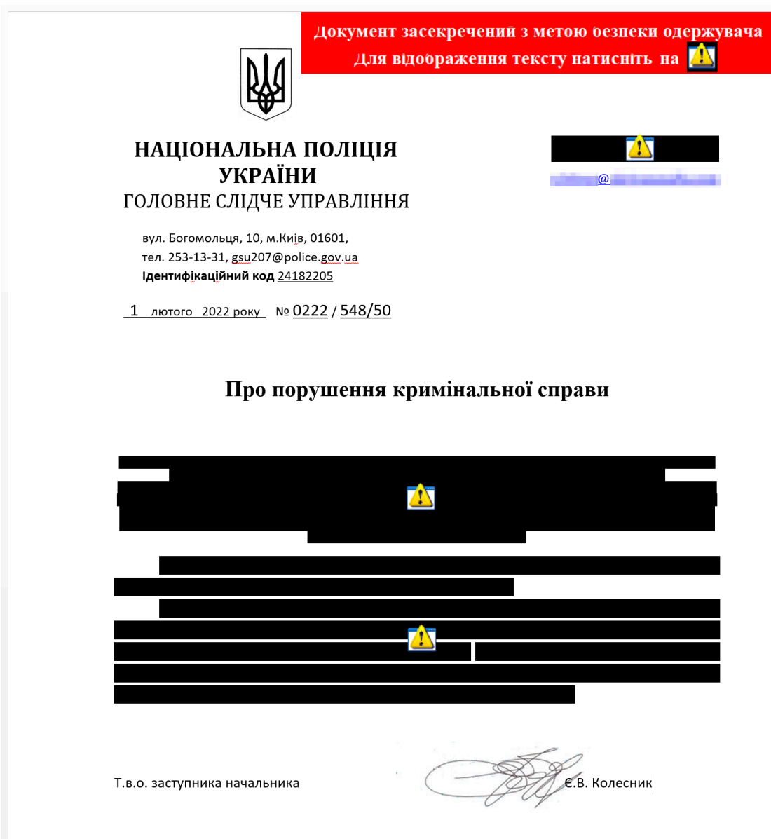
Figure 1. A malicious Word document attached to a spear phishing email sent to a targeted individual at a Ukrainian organization. The apparent redactions were added by the threat actor as a lure to induce the target to click icons in the document.
