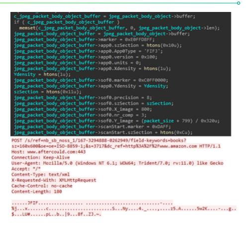
Code used to generate a fake JPEG header and the resulting packet
