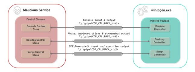
The architecture used by the attackers to stage shellcode buffers in the winlogon.exe process in order to handle various remote control features
