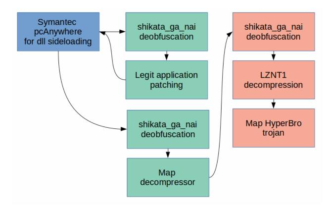
Anti-detection stages. Different colors show the three dropped modules: legit app (blue), launcher (green), and decompressor with the Trojan embedded (red)
