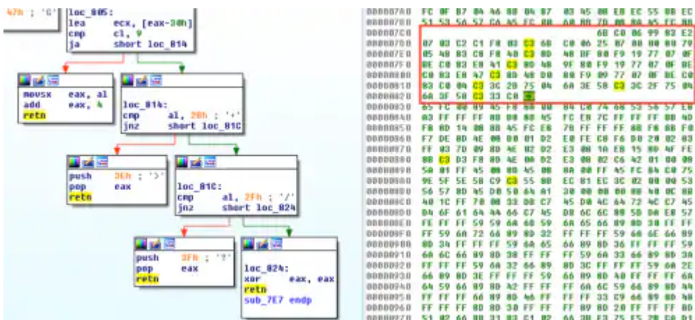
Figure 5 Additional decoding functions and associated bytes
