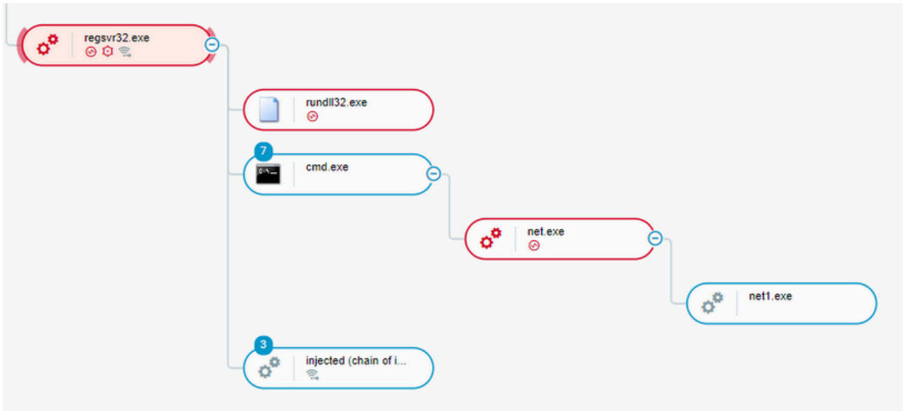
Process tree showing regsvr32.exe loading a Cobalt Strike module, executing discovery action on the network and communicating with a C2 domain
