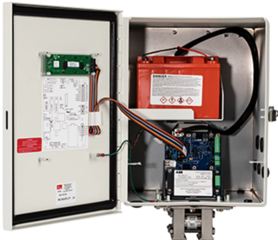
\mu FLOG5 in its enclosure. (Source: ABB)
