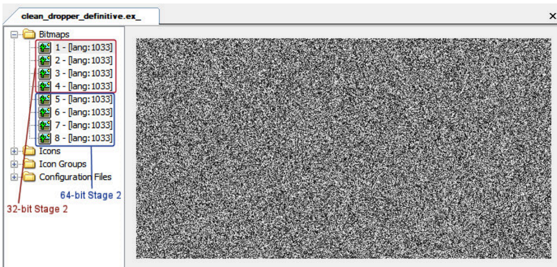
Figure 8. The fake bitmap image embedded as resource
