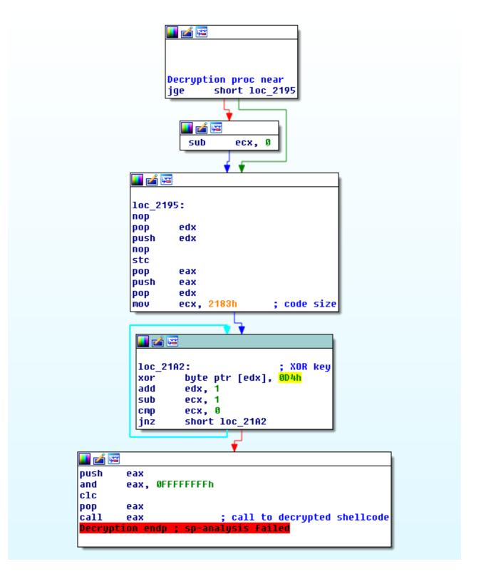
Figure 13: Decryption loop and call to decrypted shellcode
