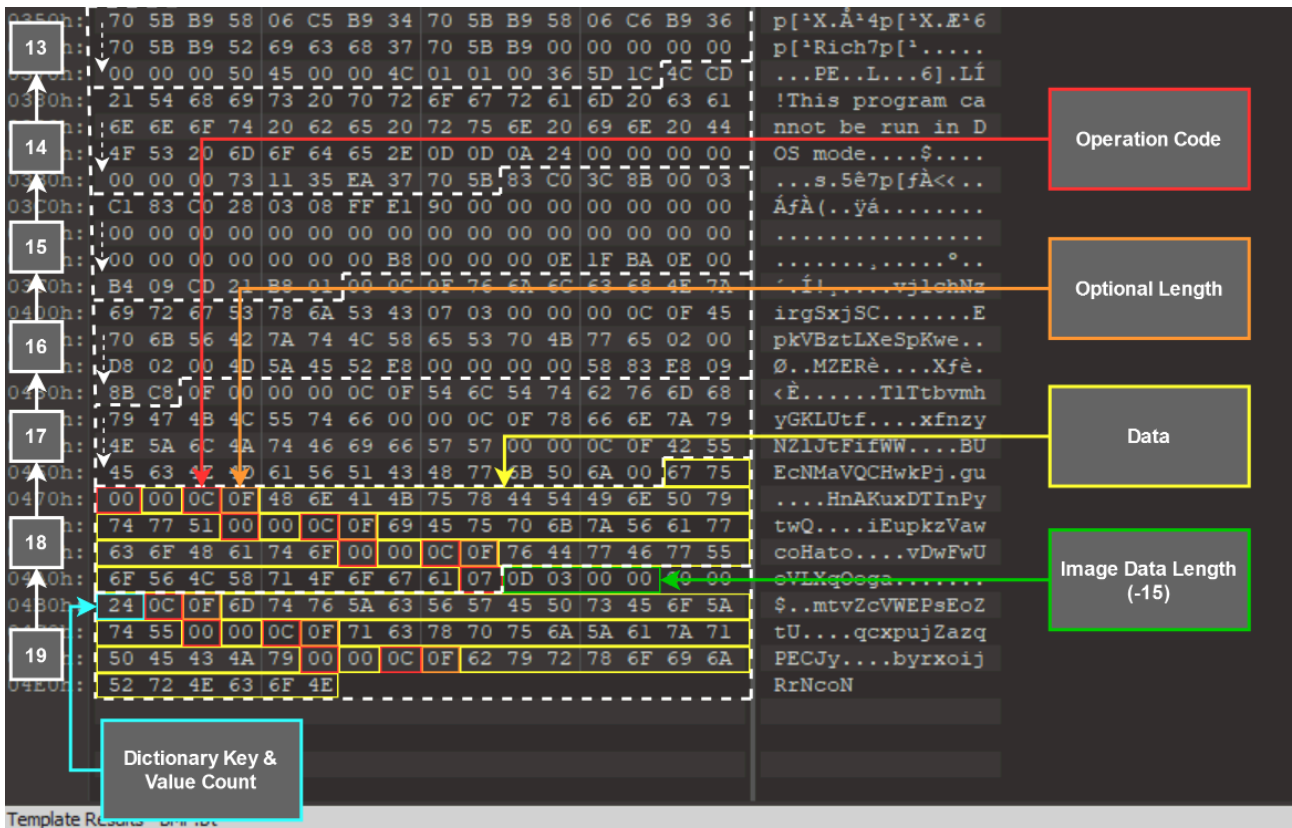
Figure 14: Partial dictionary encoded in a BMP image
