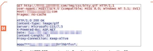
Figure 4 HTTP GET request used by Daserf to establish a session with a C2 server
