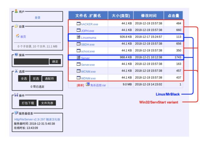
In this panel we found two instances of Linux/MrBlack along with seven instances of a variant of ServStart. We have identified the MrBlack instances based on code reuse:
