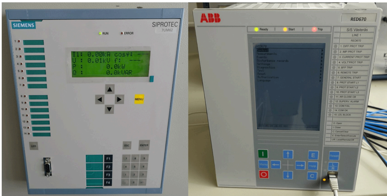
Figure 3. Protective relays for electrical substations – Industroyer spoke the language of this hardware
