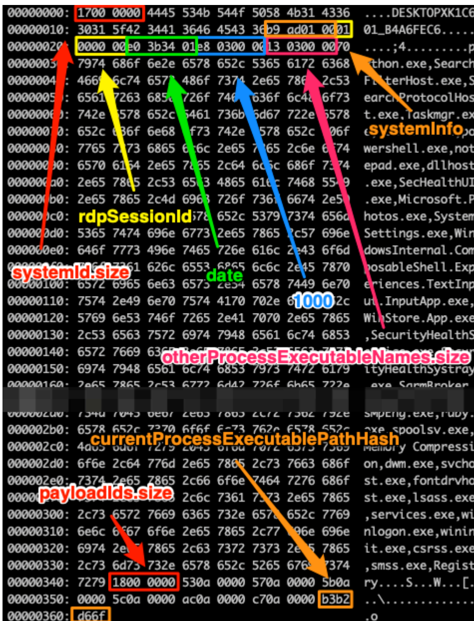
Figure 35. Emotet’s serialized request payload
