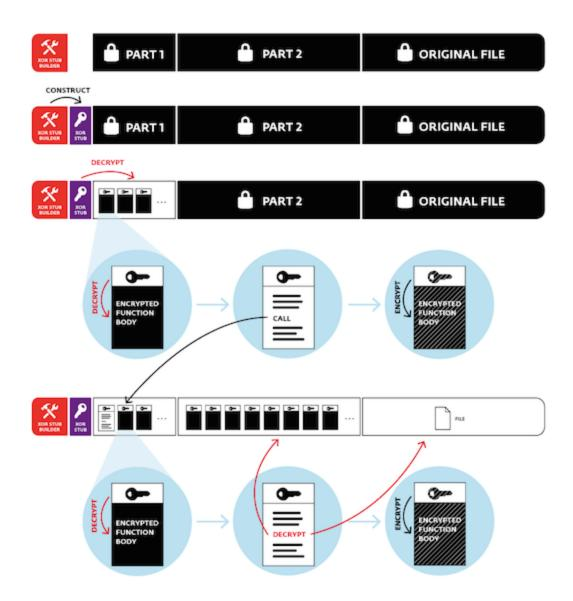
When a Win32/VirLock binary is loaded into memory, the only unencrypted code is something we'll call a *XOR stub builder*; all other code, data and the original file (if present – the same scheme applies to "stand-alone" VirLock instances) are encrypted.
